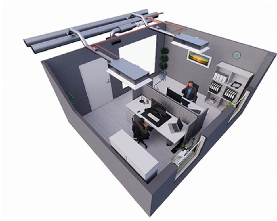
**Fig. 11:** Halton Rex RXP active chilled beams with HAQ control and PTS damper, controlled with
