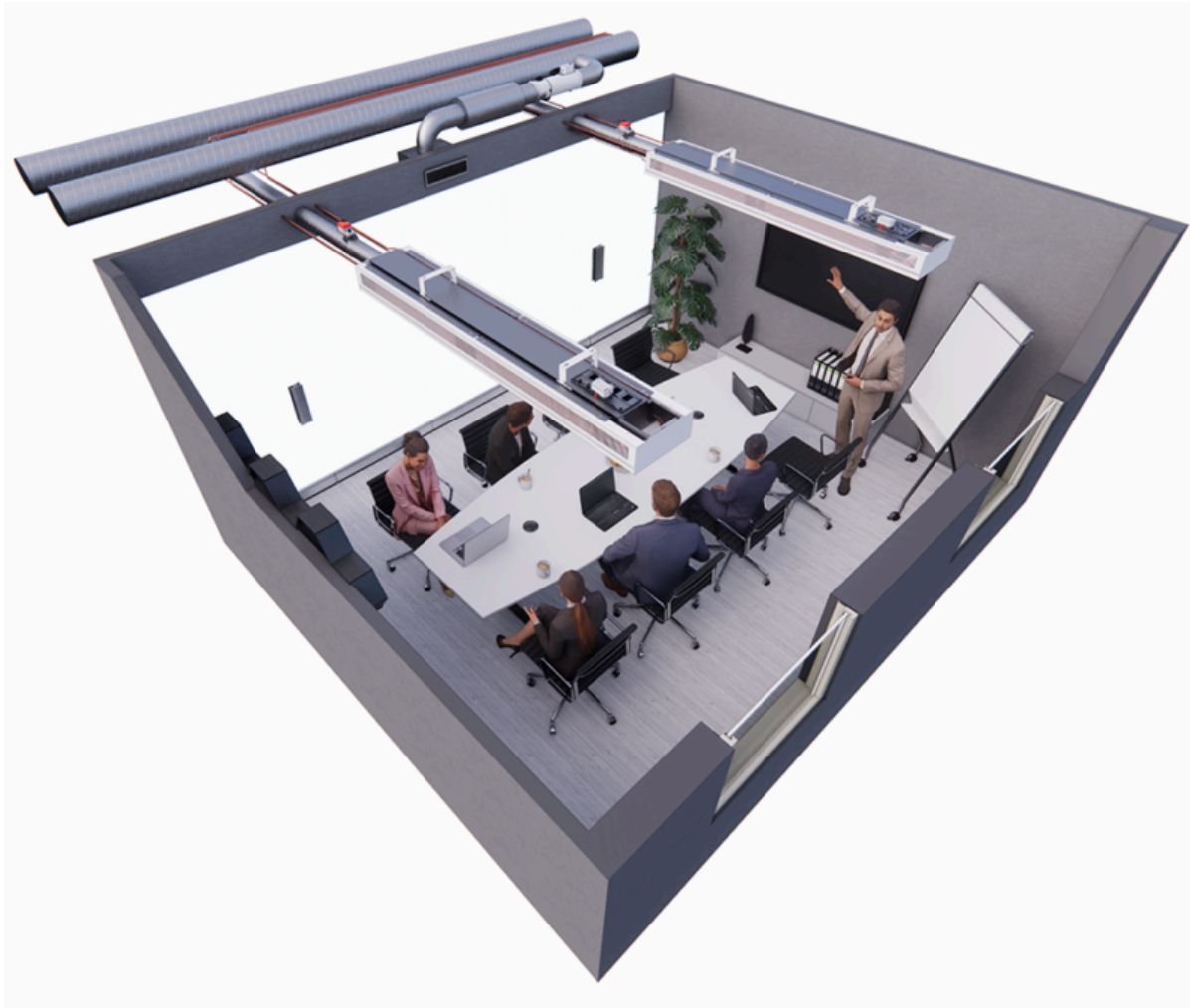
Fig. 12: Halton Rex REEactive chilled beams with HAQ control and PTS damper, controlled with Halton Workplace WRA room automation controllers in a meeting room
