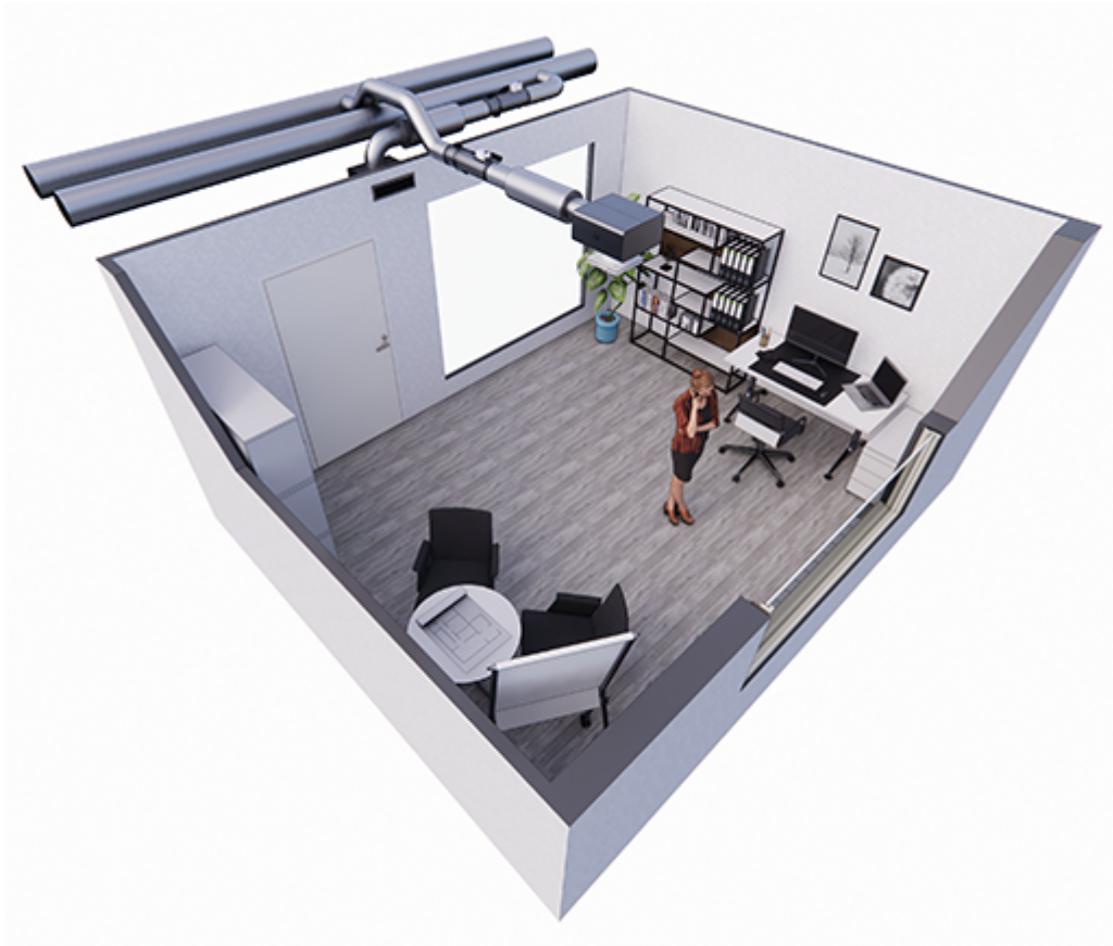
Fig.4. Halton Jaz JDA diffuser and Halton Max MUC VAV damper, controlled with Halton Workplace WRA room automation controller in a single office room
