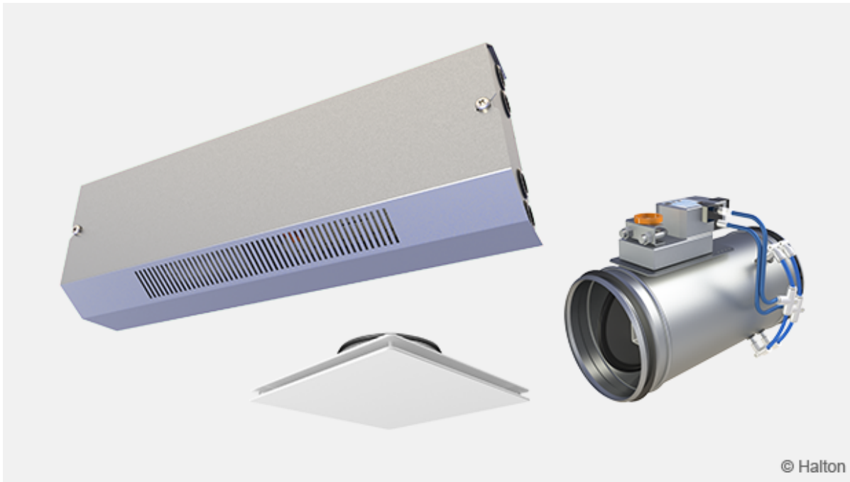
Fig.1. Halton Jaz JDA static diffuser and Halton Max One Circular VAV damper combined with a Halton Workplace room automation controller.
