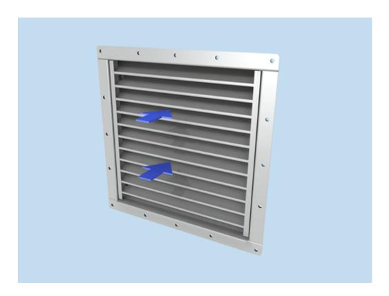
Air is supplied or extracted through the horizontal blades. The design of the grille prevents rainwater from reaching the ductwork. The slot between the frame and the top blade is sealed, ensuring rainwater doesn't enter the ductwork from above. Drops of water are collected in the grooves at the front edge of the blades, and water flows into the side grooves, where it is directed downward.
