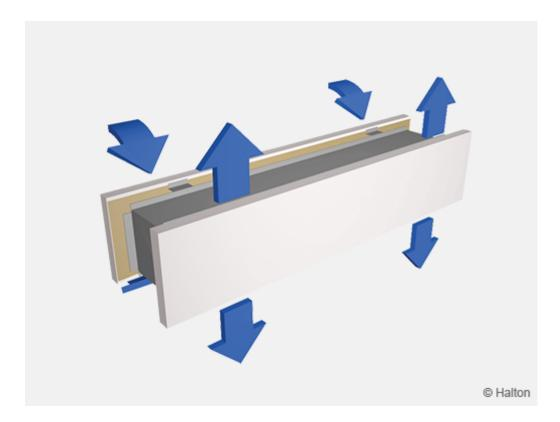
Air moves to adjoining rooms through the transfer unit due to pressure difference. The transfer unit attenuates sound and reduces air-borne noise between rooms. The transfer unit distributes air evenly in different directions. The transfer unit prevents vision from room to room.
