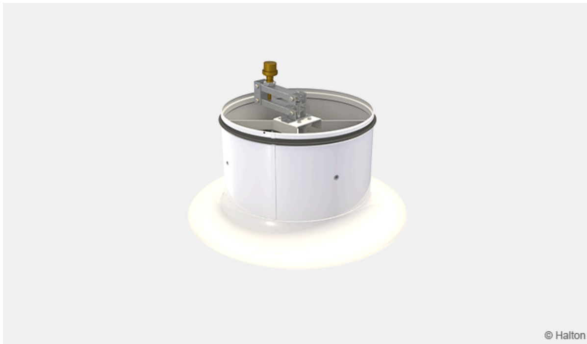
Fig.7. Halton TSA with Siemens GDB161.2E/HA actuator with 24 VAC power supply and proportional 0...10 VDC control signal
