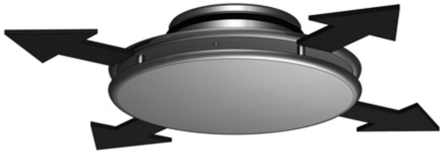
Air is supplied horizontally into the space through the side slots of the diffuser and induces the room air outside the diffuser. The recommended maximum air temperature difference between supply and room air is 10 °C degrees.
