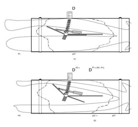
Constant airflow damper Halton RMC is an independent control element operating without an external power supply, maintaining the required airflow rate regardless of upstream pressure changes. Consequently, system balancing is not needed.
