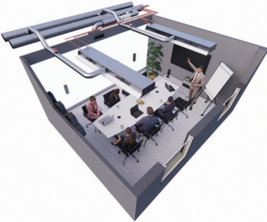
Fig. 2: Halton Rex 600 (RE6) active chilled beams with HAQ control and PTS damper, controlled with Halton Workplace WRA room automation controllers in a meeting room
