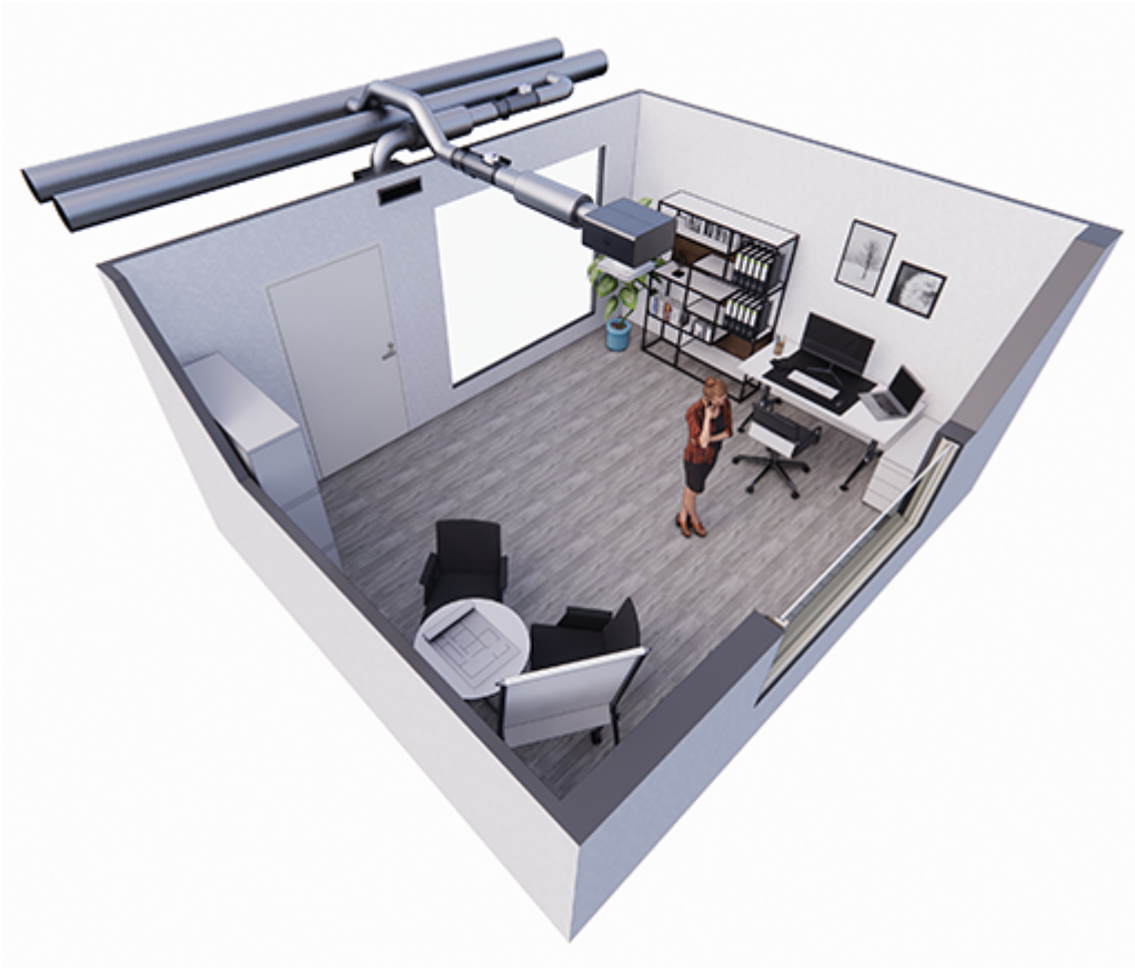
Fig.4. Halton Jaz JDA diffuser and Halton Max Ultra Circular VAV damper, controlled with Halton Workplace WRA room automation controller in a single office room
