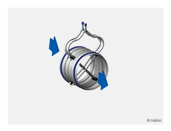
Airflow in a duct creates a pressure difference between the front and rear probes.
