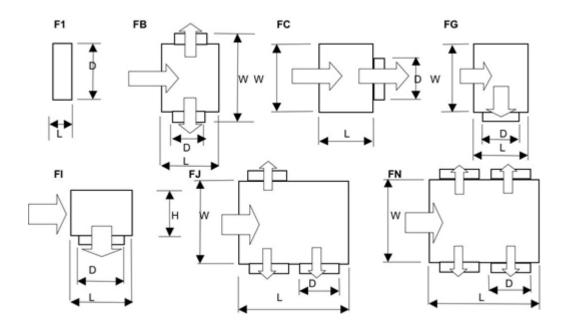
There are eight (8) different outlet connection options available for the HFD dual duct airflow management damper.
