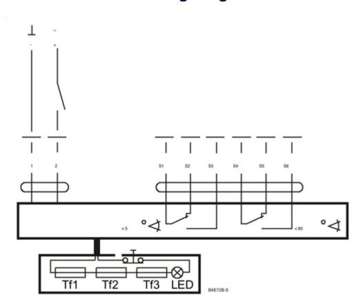
BF24-TN-2 Power supply 24 VAC/VDC (72°C) BF230-TN-2 Power supply 230 VAC (72°C)
