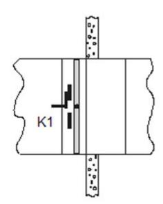
Fire damper open K1: 13/14 closed 21/22 open Fire damper closed K1: 13/14 open 21/22 closed
