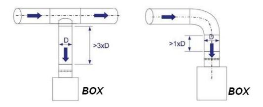
For the supply, in static pressure control, the minimum safety distance for the static measurement unit after the control damper is  $5 \times D$  in supply air applications. However, the pressure sensor position is typically halfway along or in the last third of in the last third of the duct branch length.
