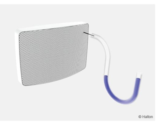
Set a probe inside the valve and measure the differential pressure with a manometer. The location for the probe would be about 20 mm from top and side surfaces.
