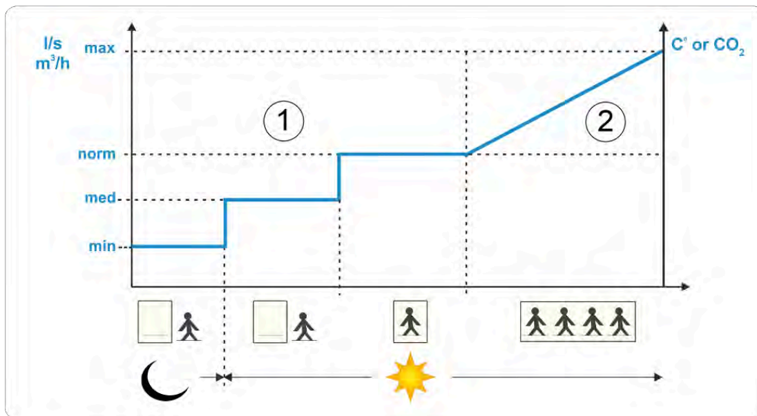
Fig. 3. Room air conditioning operating modes based on occupancy and the time of the day
