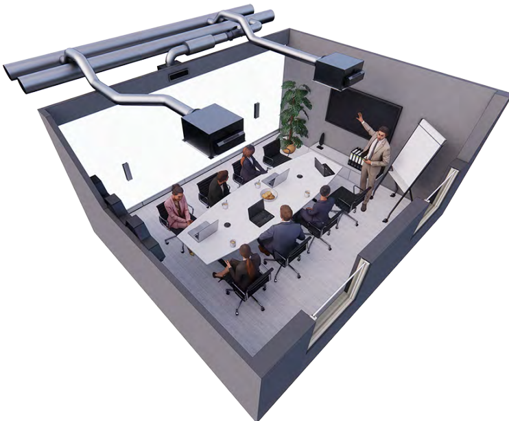
Fig. 24. Meeting room situation (boost operating mode design for a max. number of people)
