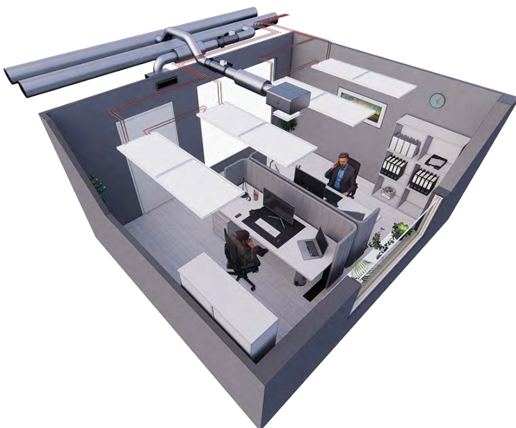
Fig. 35. Halton Jaz JDA static diffuser, Halton Max Ultra Circular (MUC) VAV damper, and Halton Ava Individual (AIN) radiant panels, controlled with a Halton Workplace WRA room automation controller in a
