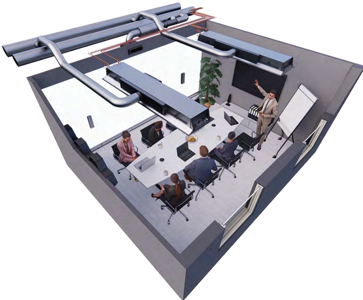
Fig. 8. Meeting room situation (boost operating mode design for a max. number of people)
