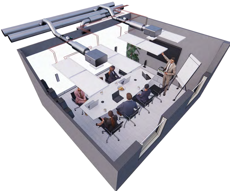
Fig. 33. Meeting room situation (boost operating mode design for a max. number of people)
