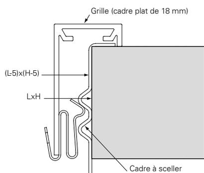
FIXATION PAR VIS APPARENTES
