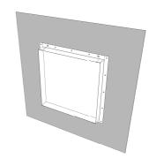
3. Apply the sealant mass to seal the fixing frame to the exhaust duct.
