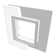
**NOTE:** While fixing the grille frame push it against the wall and pull the duct against the grille for a solid installation.
