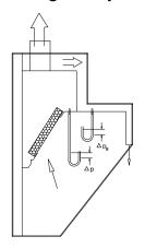
The capture jet and exhaust air flows are easily and accurately determined by measuring the pressure difference from the T.A.B.™ ports mounted in each plenum. Corresponding air flows can be read from the diagrams provided.
