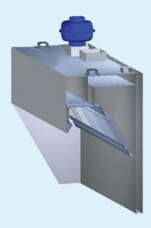
The KVL-U with Underhang model of Capture Jet<sup>TM</sup> hood is a highly efficient kitchen ventilation hood that removes contaminated air and excess heat emitted by cooking equipment, helping to provide a comfortable and clean environment.
